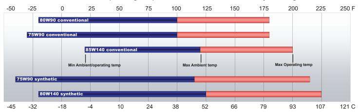
Note: Ambient temperature is the air temperature measured in the immediate vicinity of the bearing adapter. A bearing adapter exposed to the direct rays of the sun or other radiant heat sources will operate at higher temperatures and therefore must be given special consideration. The max operating temperature must not be exceeded under any circumstances, regardless of ambient temperature.
